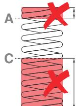
**EN** Spring rate, when verified outside the indicated range of values, may result out of the  $\pm 10\%$  tolerance.
