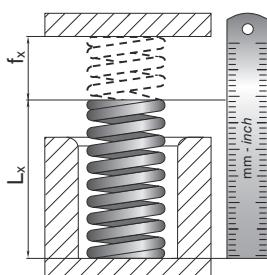
**EN** Tool maintenance can vary the original working deflection of the springs. Always check and re-set the original working stroke. Failure to do so may result in failures or damages of the tool.
