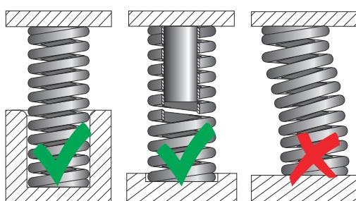
**EN** The bigger the guide the longer the lifetime. It is essential to always guide springs with a free length / diameter (L<sub>0</sub> / D<sub>H</sub>) ratio exceeding 3.5.
