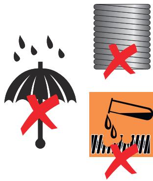
**EN** Avoid storage of springs in the fully compressed position for long periods. Protect the springs from corrosive agents to prevent oxidation and early failures. Always replace rusty springs.
