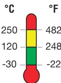
**EN** In the temperature range of 248 to 482°F (120 to 250°C) consider a loss between 1 to 2% of the load every 104°F (40°C).
