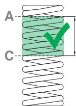
**EN** Spring rate is verified considering the force values as stated in columns A and C.
