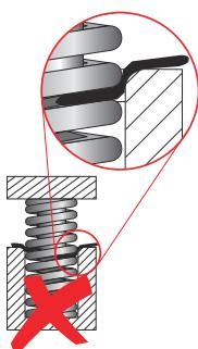
**EN** The presence of scrap or solid debris between the coils can cause a reduction of spring deflection, early failure, and damage to the tool. Check and remove scrap and debris.
