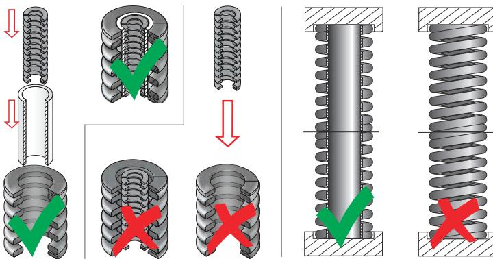
**EN** Stack springs only if guided. Coupled springs is an option provided the springs are not in contact.
